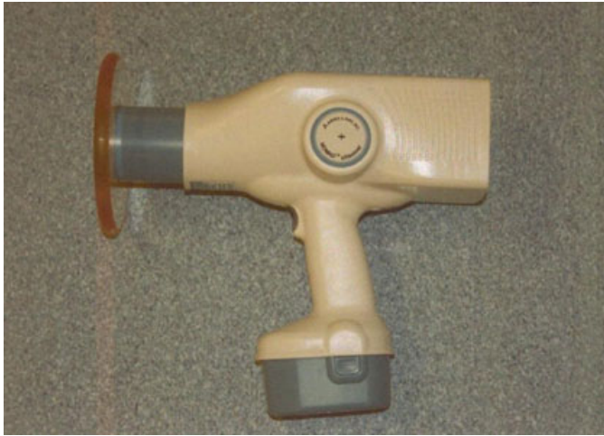
FIG. 1—The Nomad™ is a hand-held, portable X-ray unit that is powered by rechargeable batteries. It proved to be a very valuable tool in the operation at St. Gabriel.
